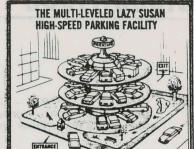
Lazy Susan facility is totally automated and computerized for fast and economical operation. When car enters at "A" and driver removes Punchcard, computer signals for an empty space. Instantly, the Lazy Susan spins and lowers or rises to produce the space.
